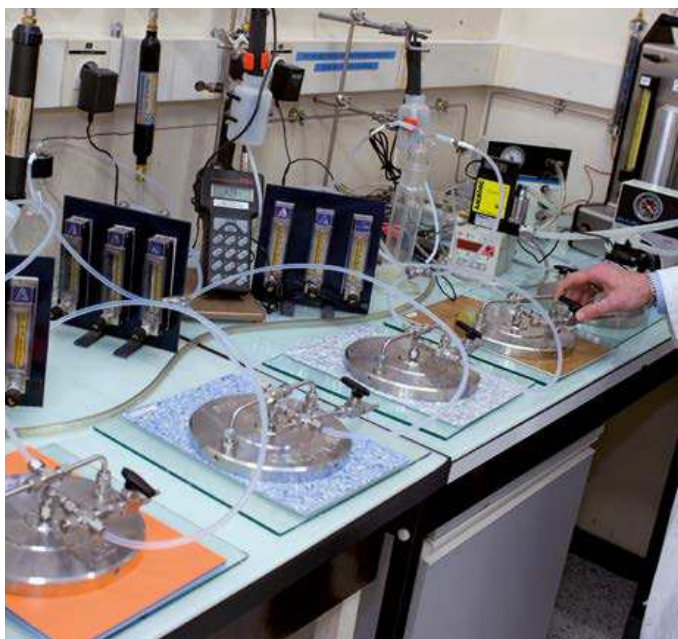
VOC emissions cell (equipment from Gerflor R&D center)
