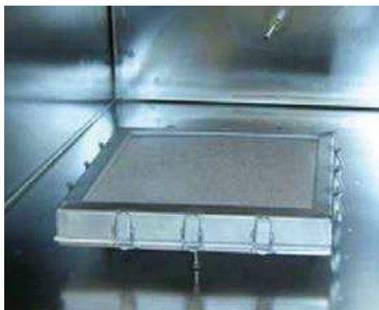
VOC emissions test chamber (used by AgBB)
